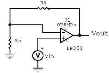
Fig. 2 Non-Inverting Amplifier Circuit
