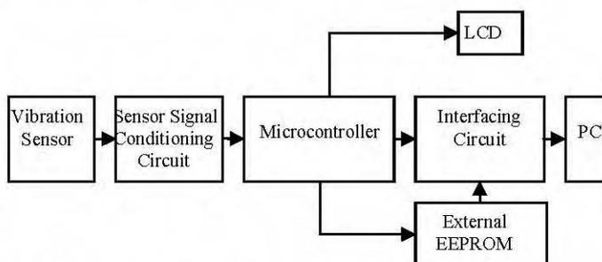
Fig. 1 Proposed Block Diagram of Seismograph for Earthquake Measurement System
