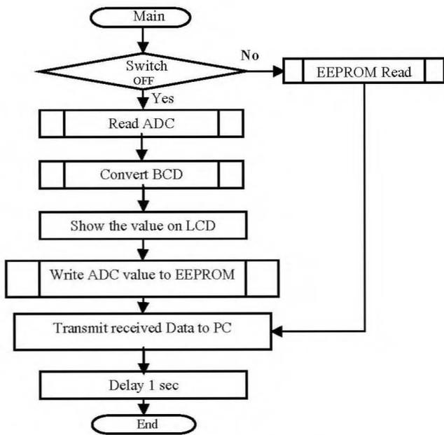
Fig. 5 Overall Flow Chart of Proposed System
