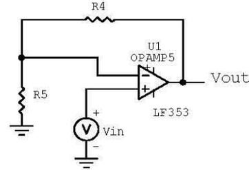
Fig. 2 Non-Inverting Amplifier Circuit
