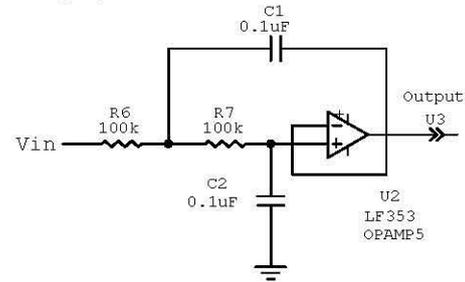
Fig. 3 Low Pass Filter Circuit
