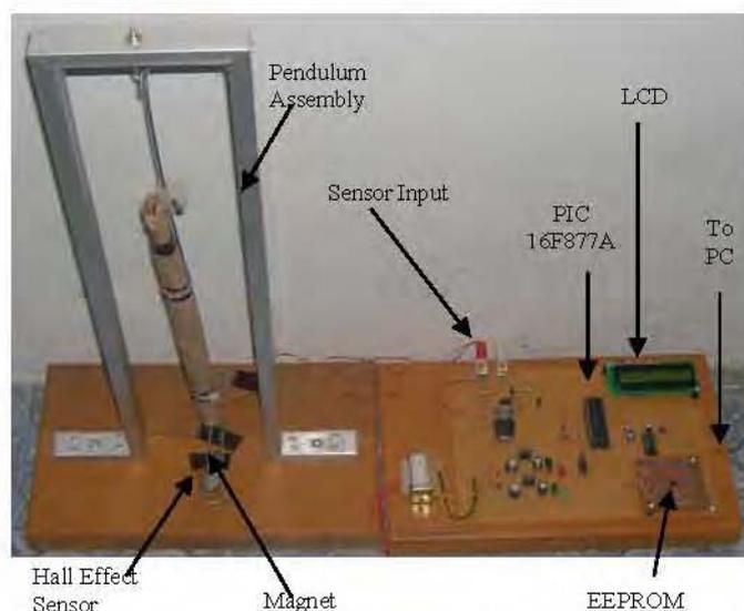
Fig. 9 Constructed Circuit Board Assemblies with the Pendulum Mechanics
