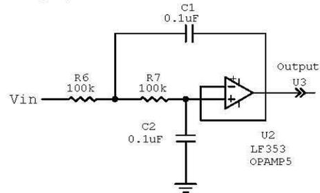
Fig. 3 Low Pass Filter Circuit
